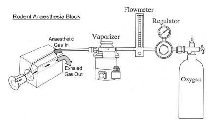
Figure 2 Diagram of a Heated Rodent Anaesthesia Block connected to an anaesthetic machine
