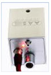
Figure 5 Close up of the ZDS Qube block. The Red light shows that heating is on. In this picture the gas ports are not connected to the anaesthetic gas delivery machine (small top port is anaesthetic gas in; the large bottom port is waste anaesthetic gas out)
