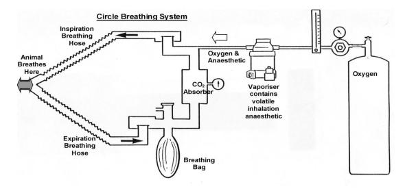
Figure 1 Diagram of an anaesthetic machine with a circle breathing system
