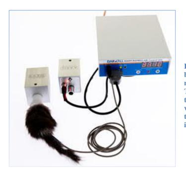
Figure 4 Shows 2 ZDS Qube. The ZDS Qu block on left shows rodent in a mask being monitored by an auxiliary temperature pro The ZDS Qube block in the centre is connec to the Heated Breathing Circuit controller which provides power and monitors the temperature of the block. The HBC control is on the right.
